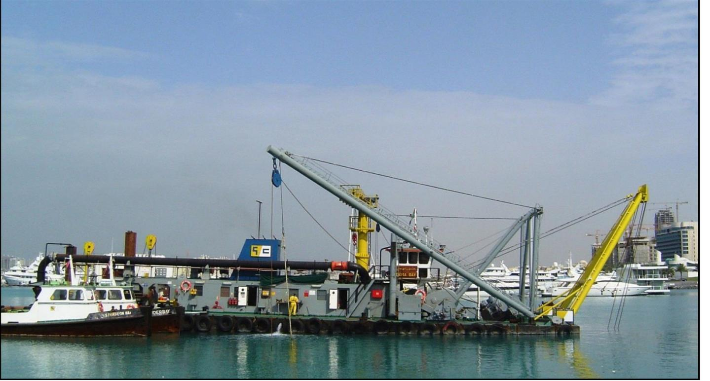
The "Deira Bay" is a medium size shallow draft cutter suction dredger, designed to dredge hard material. Years of service in a variety of materials have proven the reliability and versatility of this unit. This dredger can be economically controlled by one operator and is well instrumented to ensure optimum outputs.
